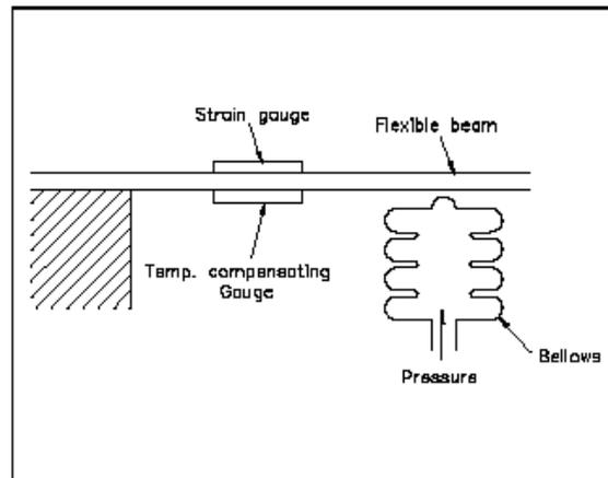
Figure 4 Strain Gauge Pressure Transducer
