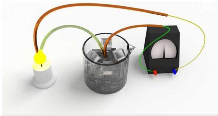
When the junctions of two metals such as copper and constantan are connected together the potential difference is produced between them. The phenomenon is called the [Seebeck effect](#) as a temperature gradient is generated along the conducting wires producing an emf. Then the output voltage from a thermocouple is a function of the temperature changes.
