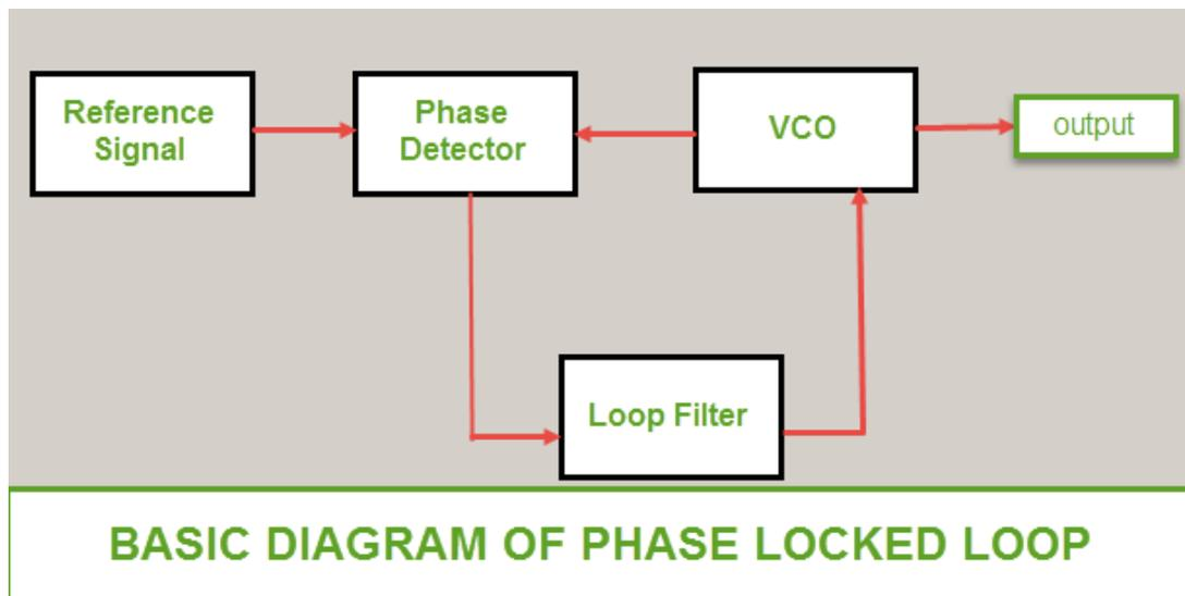
A basic phase locked loop, PLL, consists of three basic elements:
