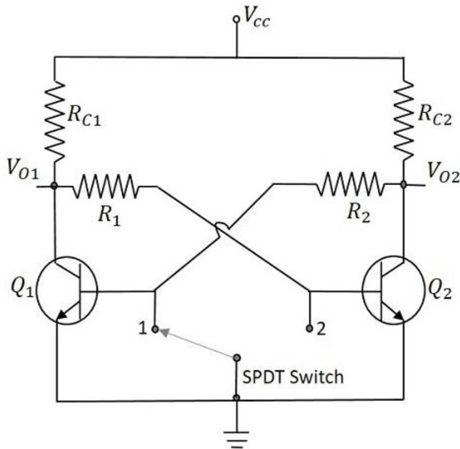
Initially we have  $Q_1$  OFF and  $Q_2$  ON. The voltage applied at the base of  $Q_2$  is  $V_{CC}$  through  $R_{C1}$  and  $R_1$ . So the output voltage will be
