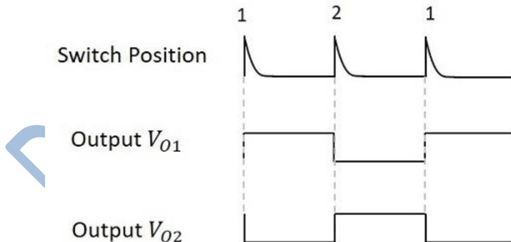
The Schmitt trigger circuit works as a **Comparator** and hence compares the input voltage with two different voltage levels called as **UTP** (Upper Trigger Point) and **LTP** (Lower Trigger Point). If the input crosses this UTP, it is considered as a
