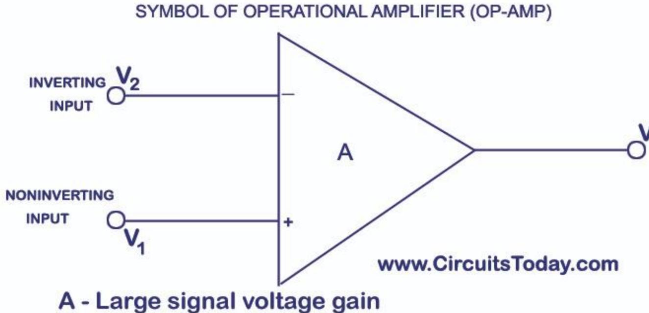
The above shown symbol is the most widely used op-amp symbol for all electronic circuits.
