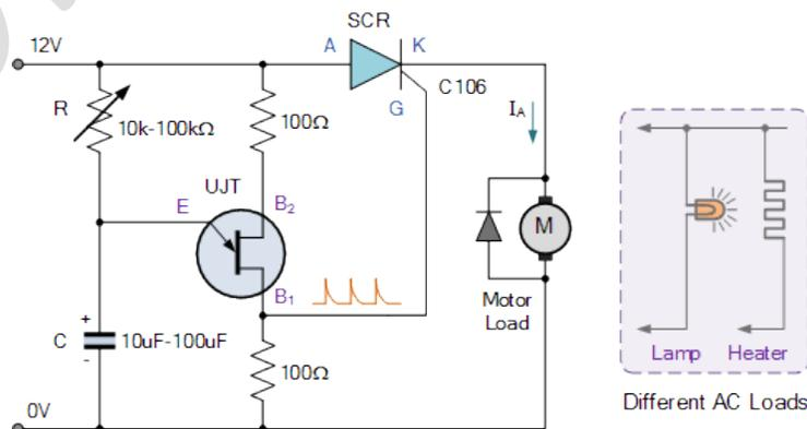
One typical application of the unijunction transistor circuit above is to generate a series of pulses to fire and control a thyristor. By using the UJT as a phase control triggering circuit in conjunction with an SCR or Triac, we can adjust the speed of a universal AC or DC motor as shown.
