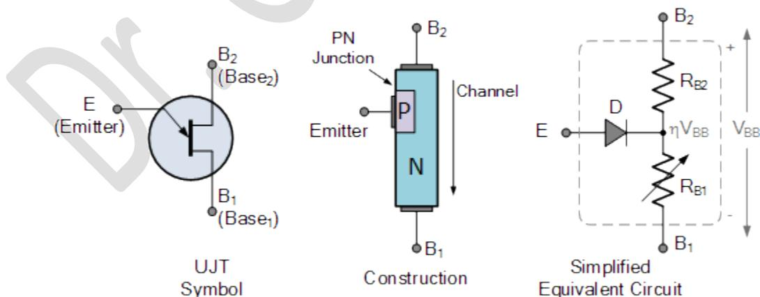
*Notice that the symbol for the unijunction transistor looks very similar to that of the junction field effect transistor or JFET, except that it has a bent arrow representing the Emitter (  $E$  )*
