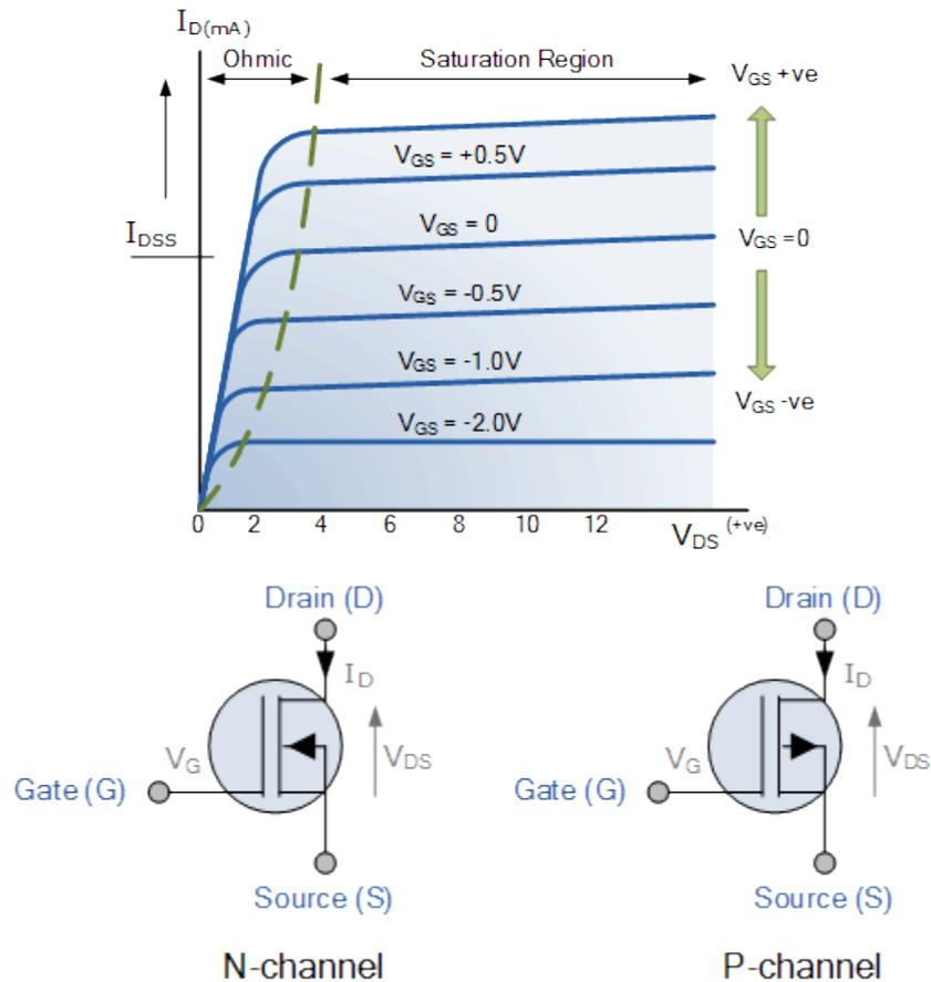
The depletion-mode MOSFET is constructed in a similar way to their JFET transistor counterparts where the drain-source channel is inherently conductive with the electrons and holes already present within the n-type or p-type channel. This doping of the channel produces a conducting path of low resistance between the Drain and Source with zero Gate bias.
