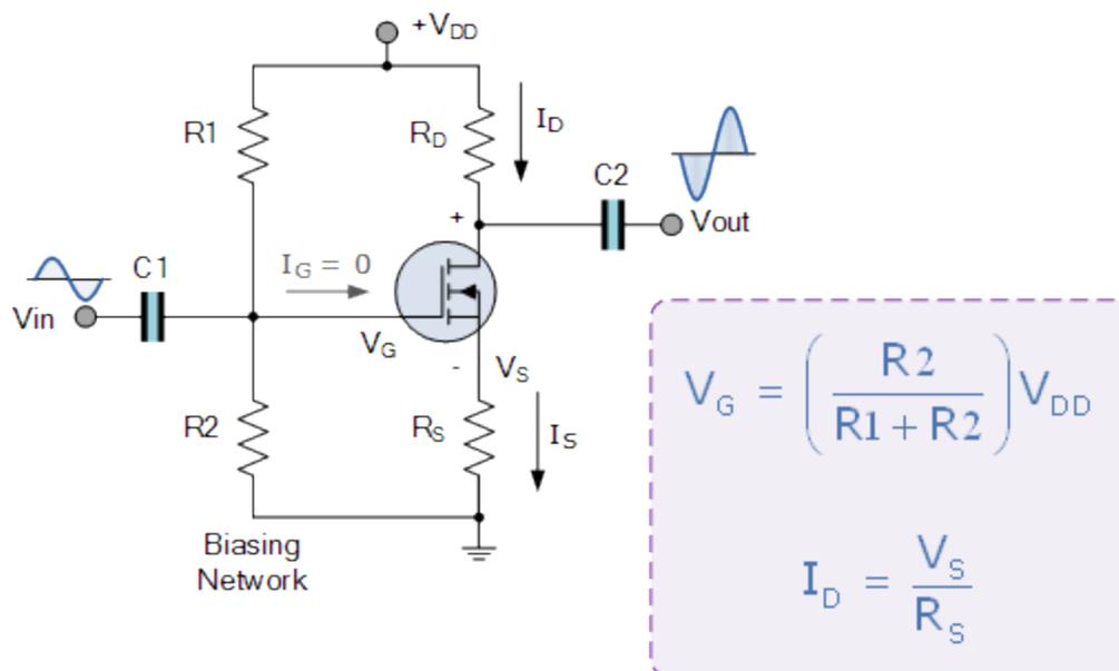
The DC biasing of this common source (CS) MOSFET amplifier circuit is virtually identical to the JFET amplifier. The MOSFET circuit is biased in class A mode by the voltage divider network formed by resistors  $R_1$  and  $R_2$ . The AC input resistance is given as  $R_{IN} = R_G = 1M\Omega$ .
