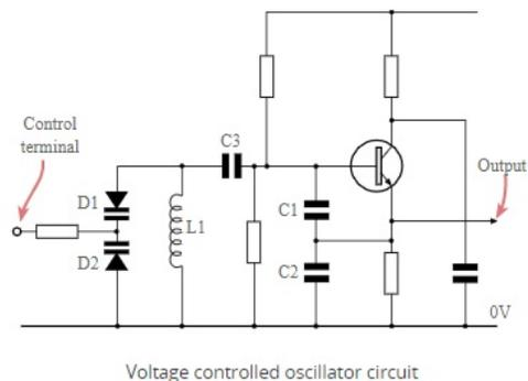
The resonant circuit is made by including an inductive element between the base and ground. In the Colpitts circuit this consists of just an inductor, whereas in the Clapp circuit an inductor and capacitor in series are used.
