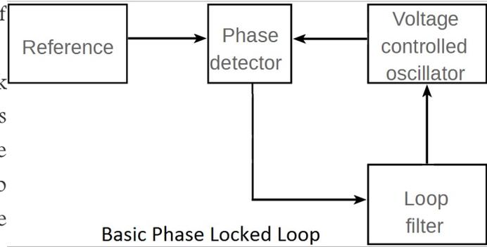
**Voltage controlled oscillator (VCO):** The voltage controlled oscillator is that part of the circuit that generates the output signal. Its frequency can be controlled over the operational frequency band of the feedback loop with help of a dc input voltage signal (which is provided by the phase comparator through the loop filter).
