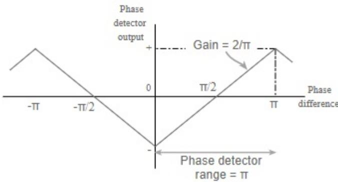
The characteristic of the phase detector is as shown in the adjacent figure. One can see that within the range of  $\pm\pi$ , the phase detector output is a linear function of phase difference.
