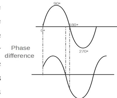
When two signals have different frequencies it is found that the phase difference between the two signals is always varying. The reason for this is that the time for each cycle is different and accordingly their phases are changing at different rates.
