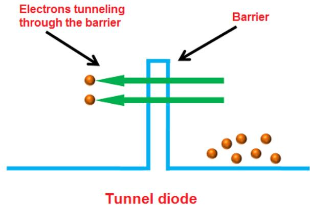
According to Quantum mechanics, the electrons directly penetrate through the depletion layer or barrier if the depletion width is very small. The depletion layer of tunnel diode is very small. It is in nanometers. So the electrons can directly tunnel across it from n-side conduction band into the p-side valence band.
