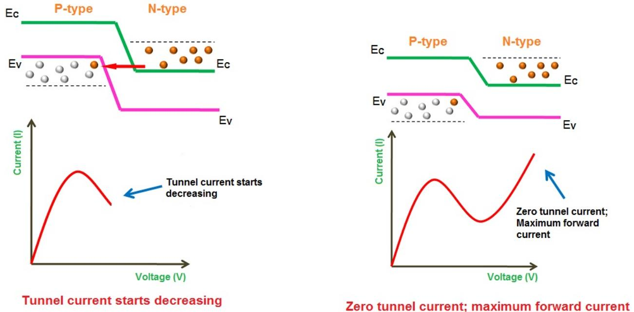
The portion of the curve in which current decreases as the voltage increases is the negative resistance region of the tunnel diode. The negative resistance region is the most important and most widely used characteristic of the tunnel diode. A tunnel diode operating in the negative resistance region can be used as an amplifier or an oscillator.
