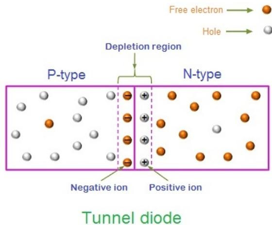
Tunnel Diodes are generally constructed from Germanium. But they are also made from other types of materials such as gallium arsenide, gallium antimonide, and silicon.
