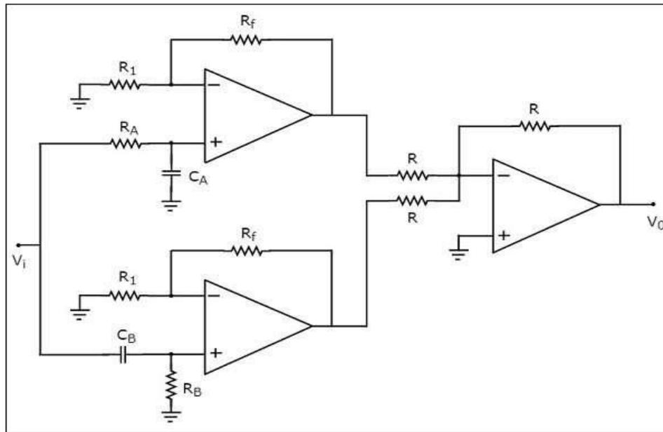
We have already seen the circuit diagrams of an active low pass filter, an active high pass filter and a summing amplifier. Observe that we got the above circuit diagram of active band stop filter by replacing the blocks with the respective circuit diagrams in the block diagram of an active band stop filter.
