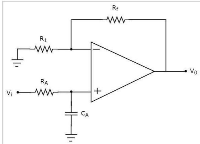
We know that the electric network, which is connected to the non-inverting terminal of an op-amp is a **passive low pass filter**. So, the input of a non-inverting terminal of an op-amp is the output of a passive low pass filter.
