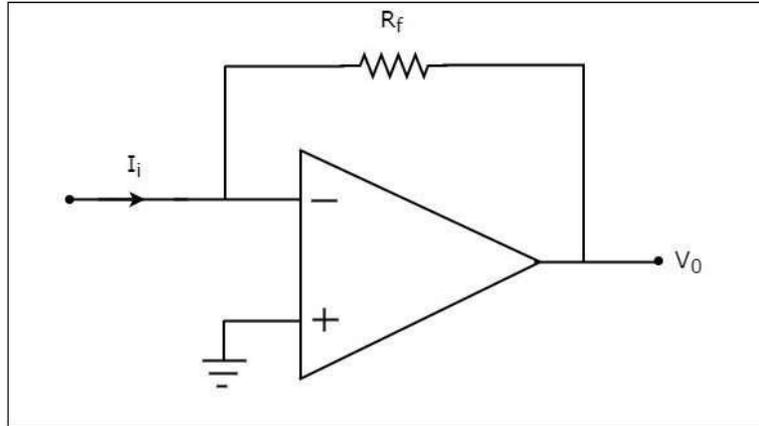
In the circuit shown above, the non-inverting input terminal of the op-amp is connected to ground. That means zero volts is applied at its non-inverting input terminal. According to the virtual short concept, the voltage at the inverting input terminal of an op-amp will be equal to the voltage at its non-inverting input terminal. So, the voltage at the inverting input terminal of the op-amp will be zero volts.
