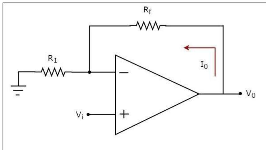
In the circuit shown above, an input voltage  $V_i$  is applied at the non-inverting input terminal of the op-amp. According to the virtual short concept, the voltage at the inverting input terminal of an op-amp will be equal to the voltage at its non-
