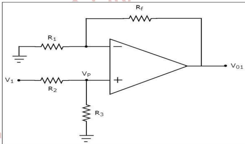
Now, using the voltage division principle, calculate the voltage at the non-inverting input terminal of the op-amp.
