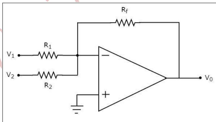
In the above circuit, the non-inverting input terminal of the op-amp is connected to ground. That means zero volts is applied at its non-inverting input terminal.
