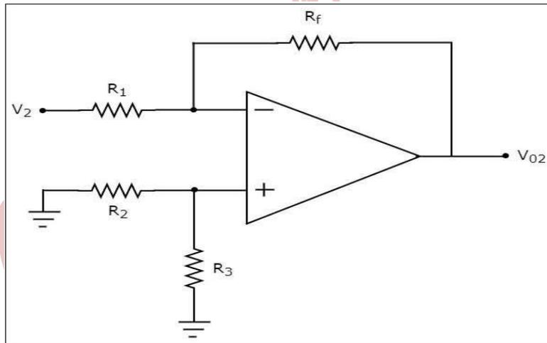
You can observe that the voltage at the non-inverting input terminal of the op-amp will be zero volts. It means, the above circuit is simply an inverting op-amp. Therefore, the output voltage  $V_{02}$  of above circuit will be –
