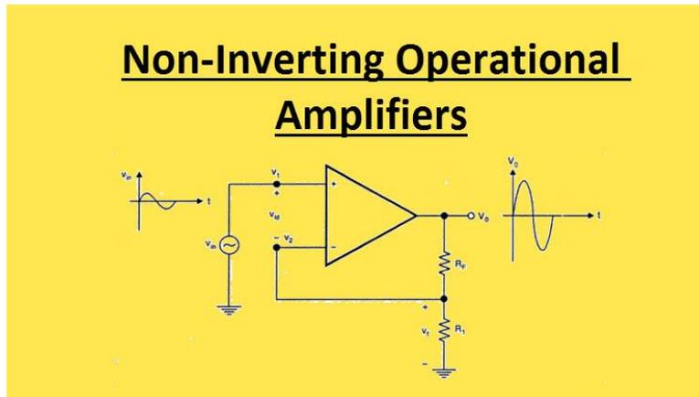
By applying an input signal to the non-inverting input and negative feedback to the inverting input, it is possible to design a circuit that does not invert the sense of the input signal.
