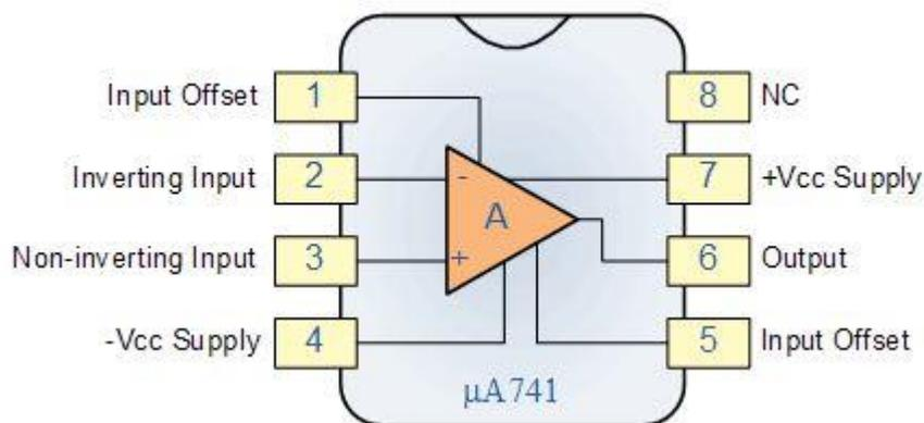
**Non-inverting input:** The operational amplifier non-inverting input is marked by a "+" sign on the circuit diagram. It is found that a positive voltage applied to the non-inverting input will produce a positive swing at the output. If a changing waveform, such as a sine wave is applied to the non-inverting input, then it will appear in the same sense at the output. It has not been inverted.
