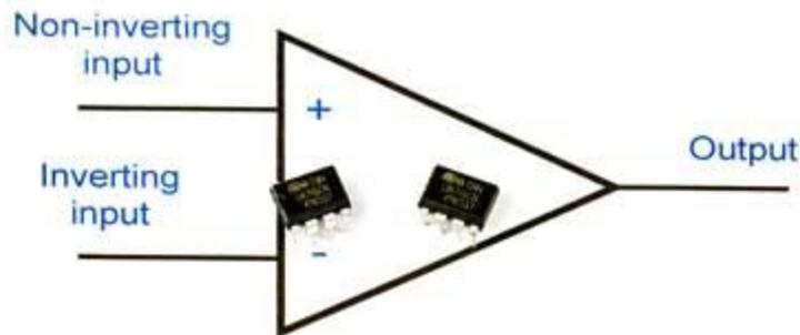
Fig: Operational amplifier circuit symbol with ICs
