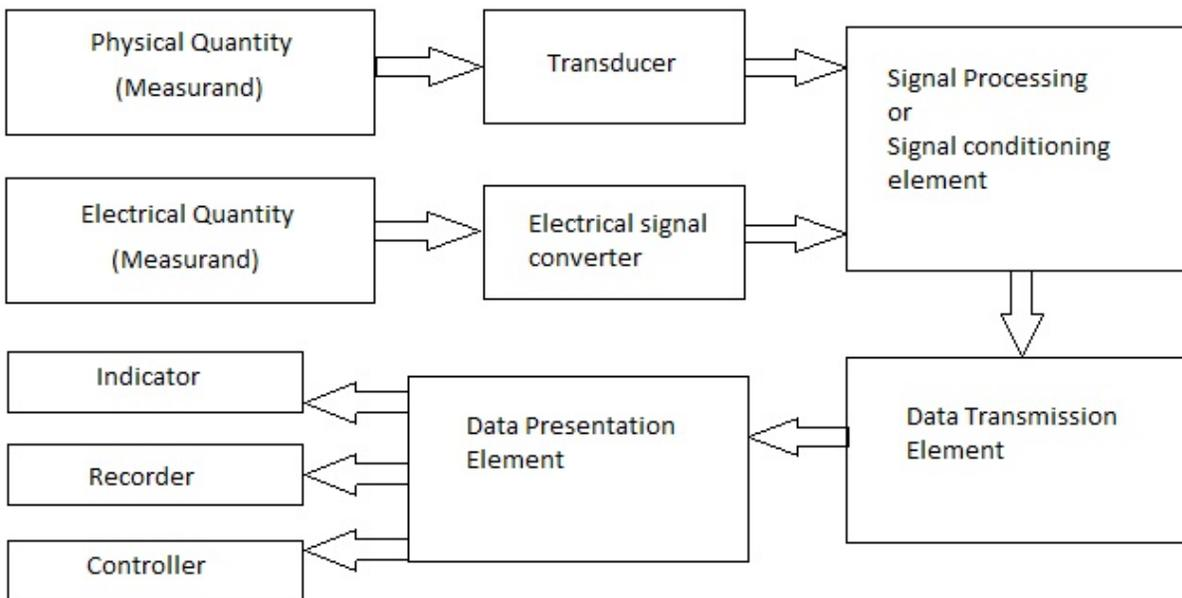
Block Diagram of a General Instrumentation System
