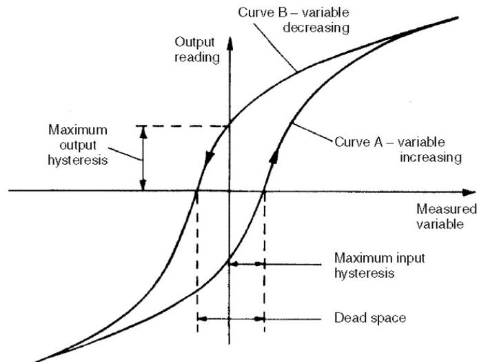
**Hysteresis:** In some instruments, the readings for the same magnitude of the measurand are different when it is increasing and when it is decreasing. The reading appears to lag behind the actual value as shown in the figure. This lagging behind is called hysteresis.
