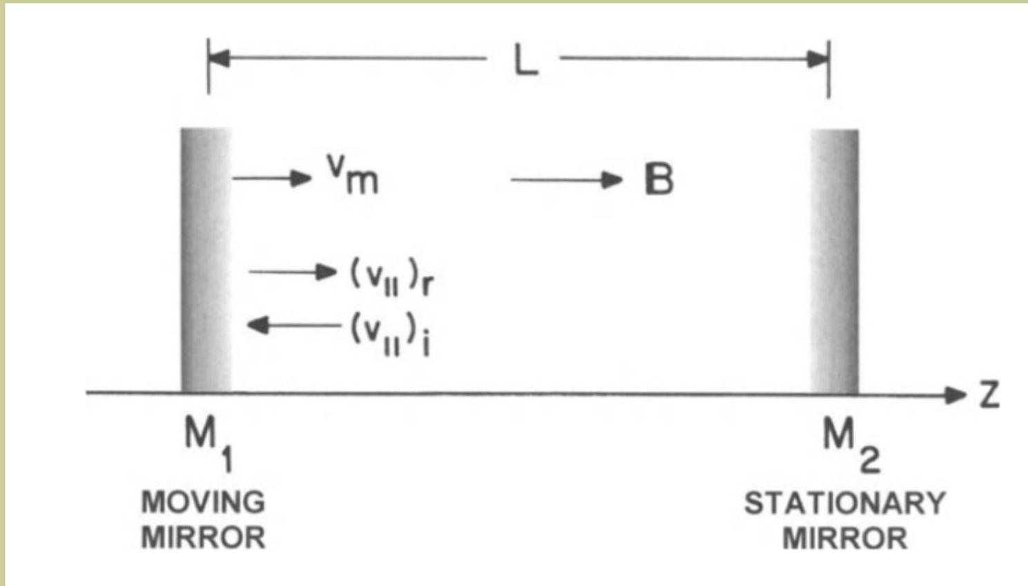
*Schematic representation of a system of two coaxial magnetic mirrors approaching each other. The figure is taken from the "Fundamentals of the Plasma Physics" by Bittencourt.*
