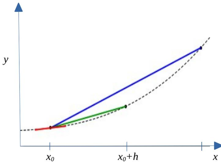
Let's assume that the dashed curve in the above figure represents the actual solution  $y(x)$  between  $x_0 < x < x_0+h$ . Now we draw a secant line between  $x=x_0$  and  $x=x_0+h$  on the curve. For different  $h$  values, we get different secant lines shown in color blue, green and red in the above figure. It is evident that for a smaller value of  $h$ , the secant line approximately represents the tangent of the curve at  $x=x_0$  point. Therefore, for a small value of  $h$ ,
