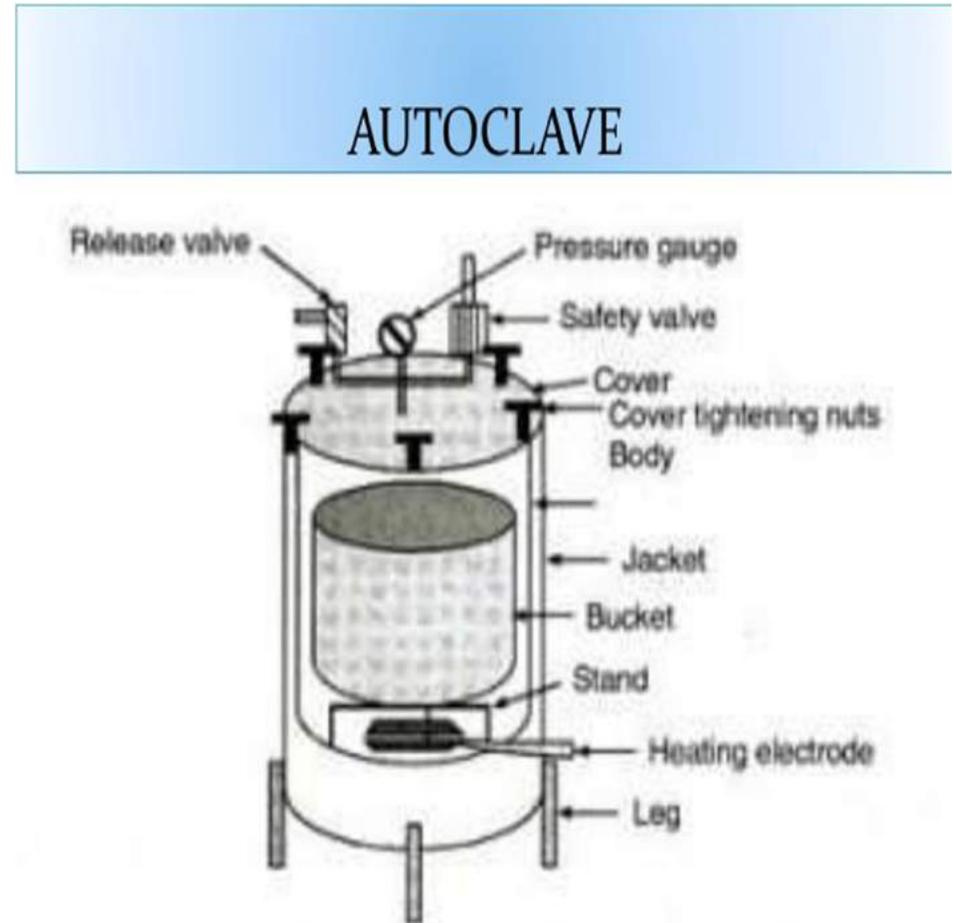
Fig. 25.2. A schematic diagram of laboratory autoclave.
