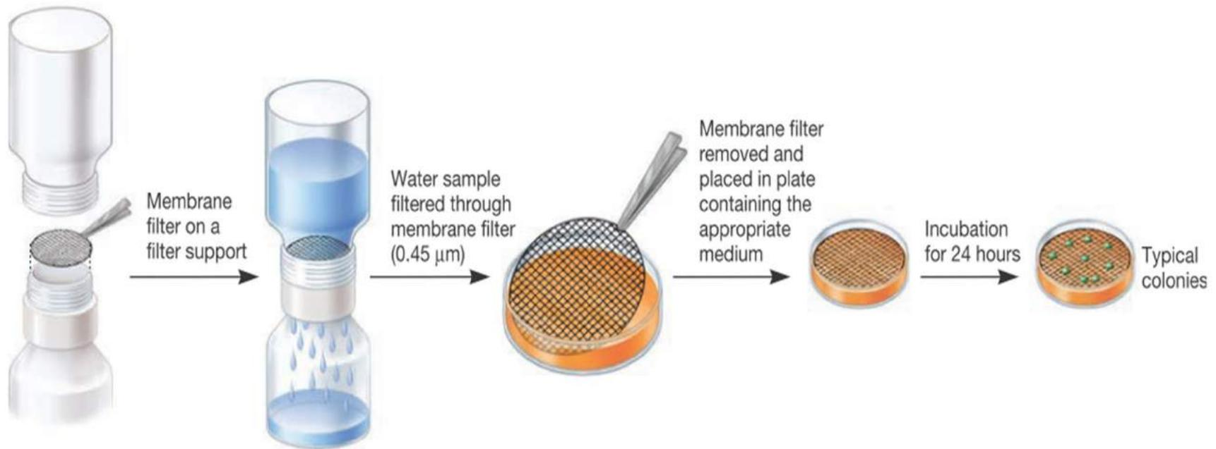
**Figure 6.13 The Membrane Filtration Procedure.** Membranes with different pore sizes are used to trap different microorganisms. Incubation times for membranes also vary with the medium and microorganism.
