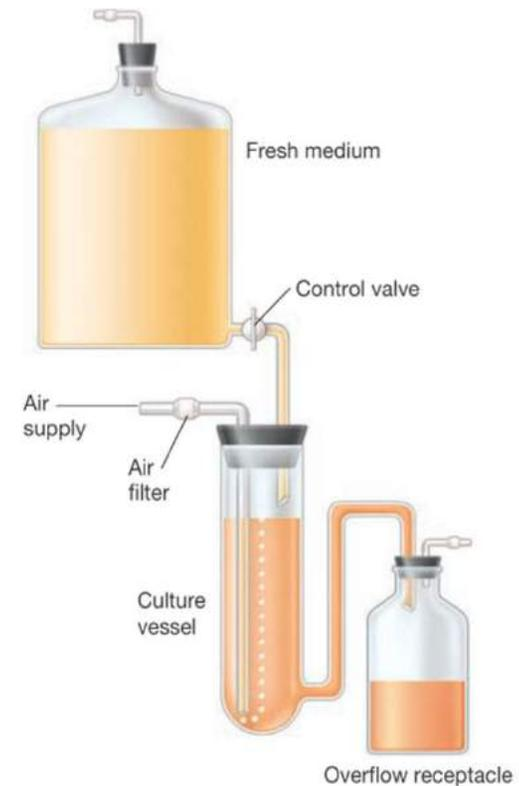
**Figure 6.16** A Continuous Culture System: The Chemostat. Schematic diagram of the system. The fresh medium contains a limiting amount of an essential nutrient. Growth rate is determined by the rate of flow of medium through the culture vessel.
