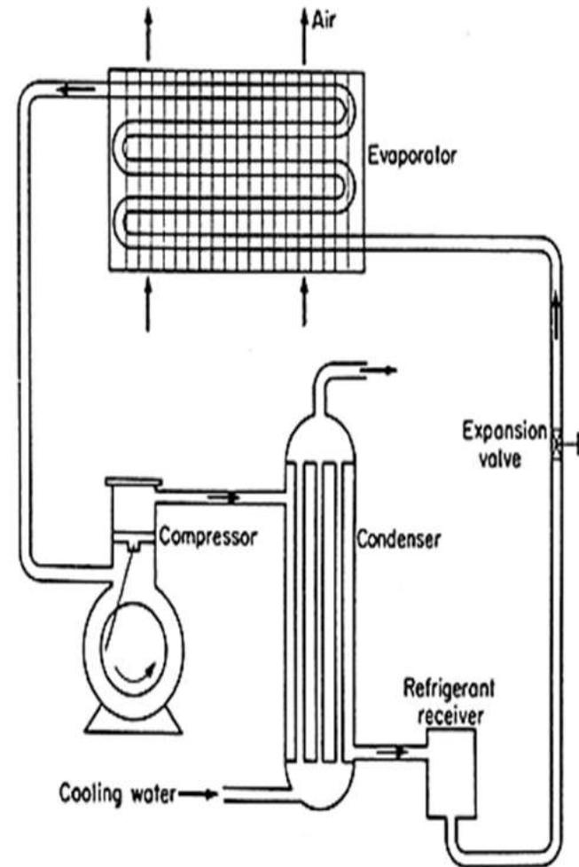
Fig- Mechanical refrigeration circuit
