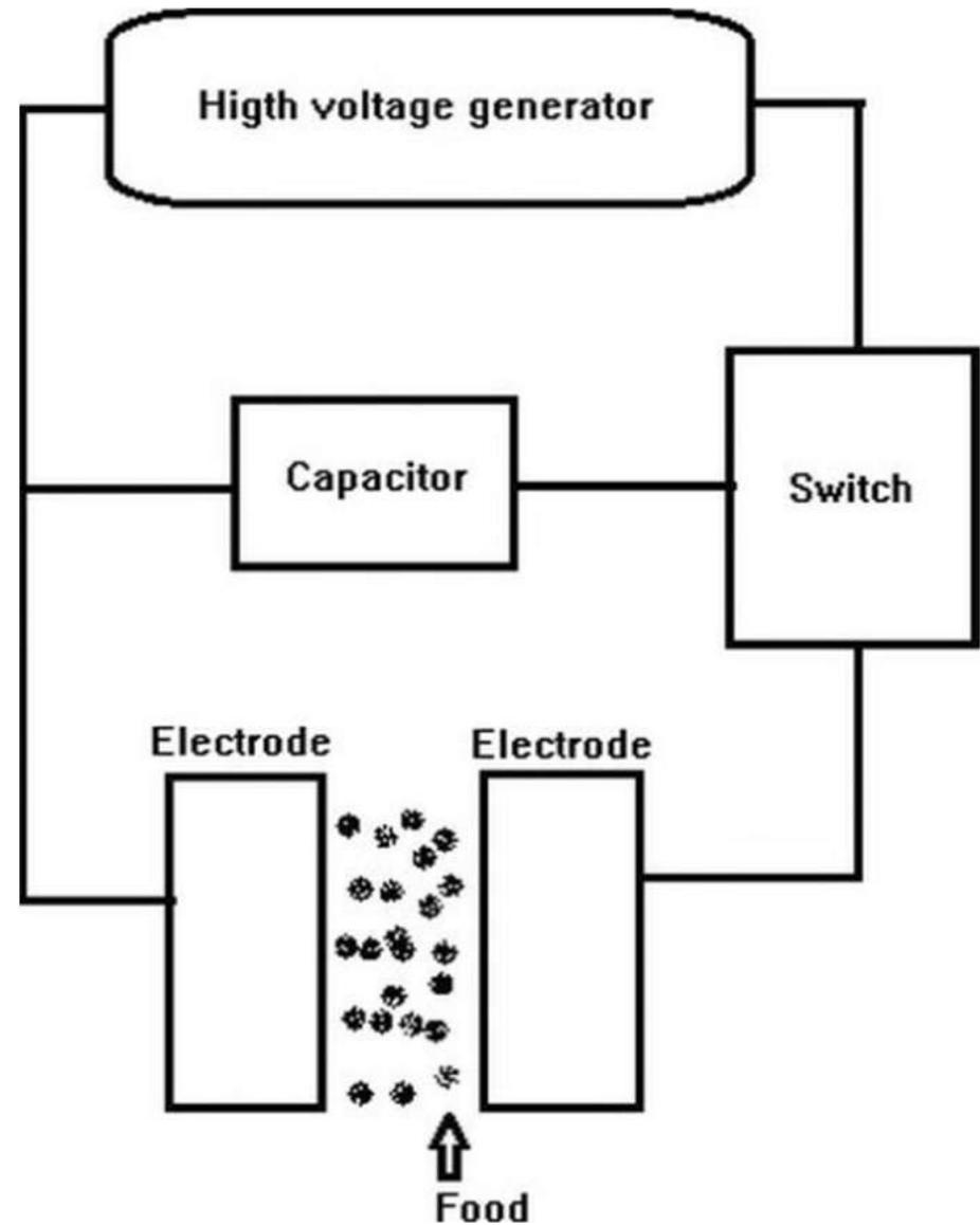
Fig: Pulsed electrical field technology
