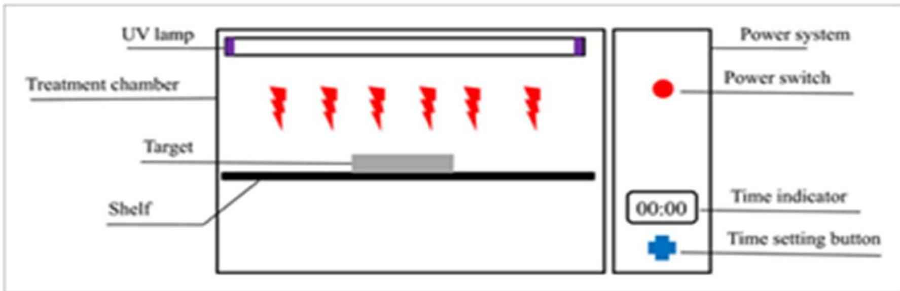
Fig: Diagram of a pulsed UV light system for treating food stuff (From - Google)
